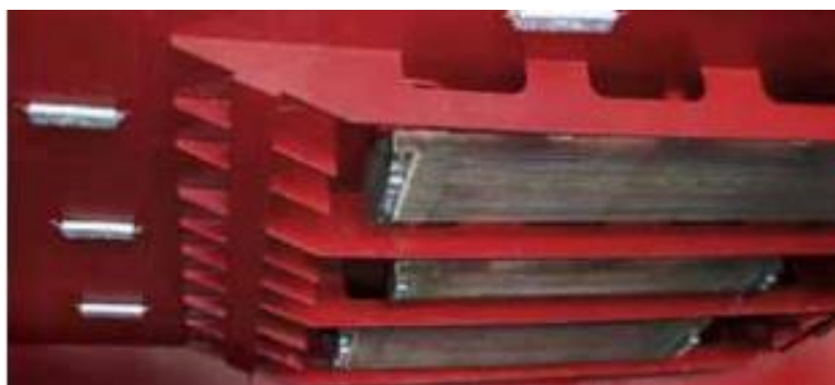
Figure 7: External Mounted Keel Cooler with Guards
